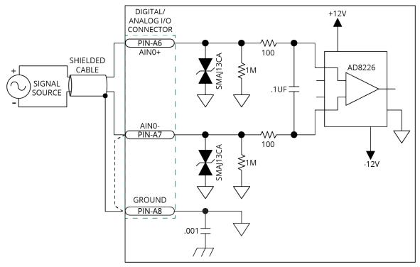
Figure 2-22: Analog Inputs Schematic
