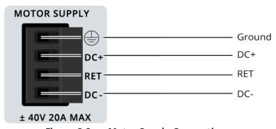
Figure 2-2: Motor Supply Connections
