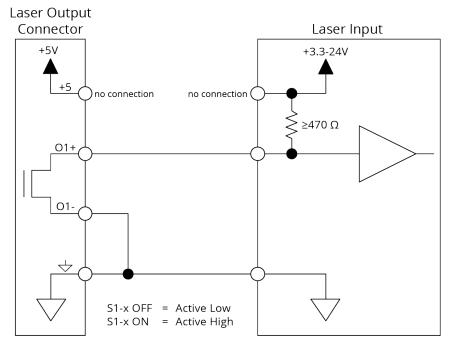
Figure 2-7: Current Sinking Configuration without Isolation
