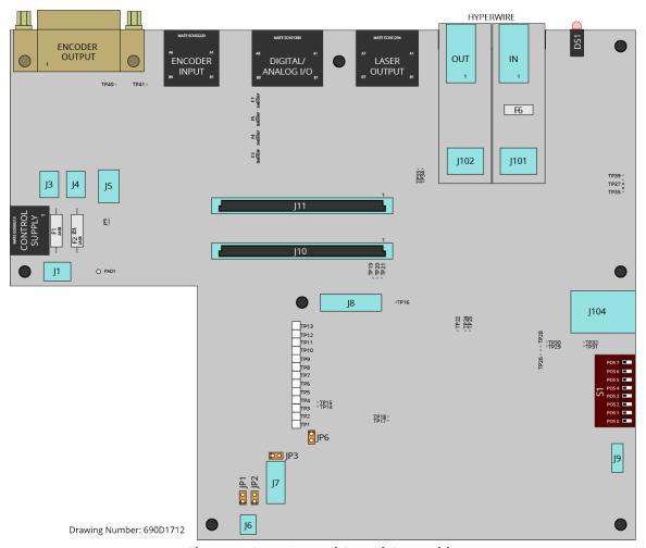
Figure 3-1: Control Board Assembly
