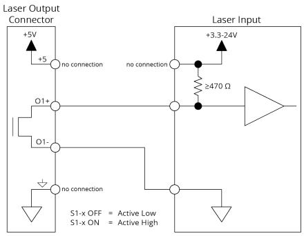
Figure 2-6: Current Sinking Configuration with Isolation
