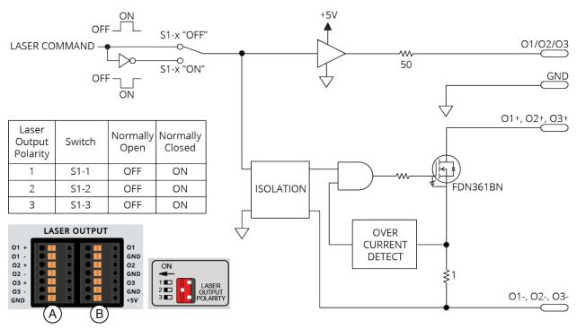
Figure 2-5: Laser Interface Outputs
