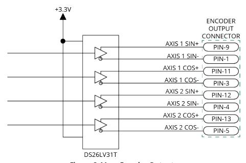
Figure 2-11: Encoder Outputs
