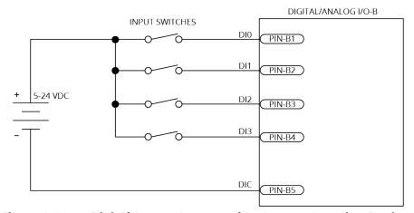
Figure 2-20: Digital Inputs Connected to Current Sourcing Devices
