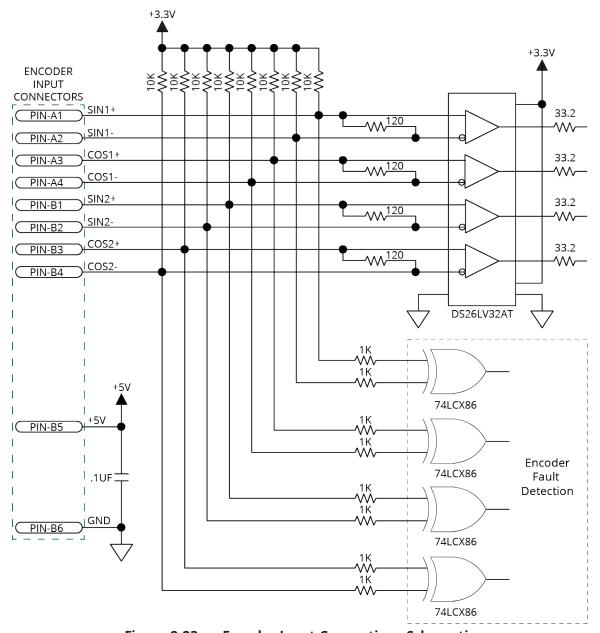
Figure 2-23: Encoder Input Connections Schematic
