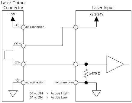
Figure 2-8: Current Sourcing Configuration with Isolation
