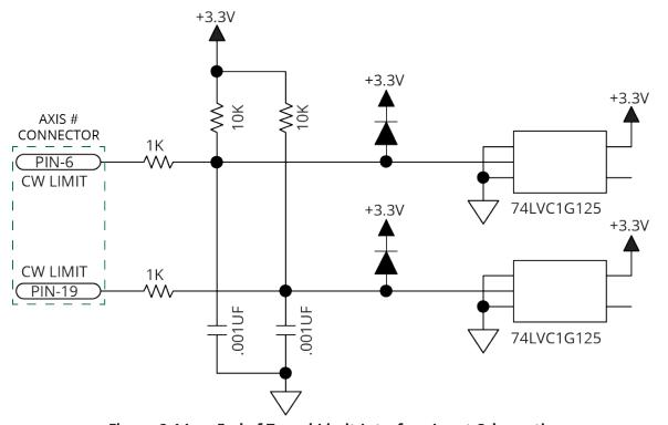
Figure 2-14: End of Travel Limit Interface Input Schematic
