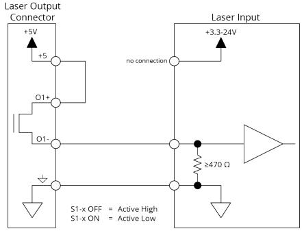
Figure 2-9: Current Sourcing Configuration without Isolation
