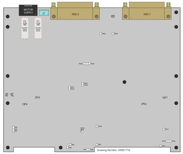
Figure 3-2: Power Board Assembly
