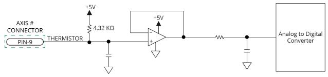
Figure 2-16: Thermistor Input Input Schematic
