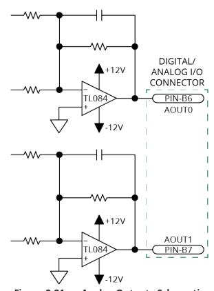
Figure 2-21: Analog Outputs Schematic
