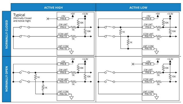
Figure 2-13: End of Travel Limit Input Connections
