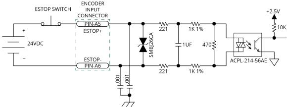
Figure 2-24: ESTOP Sense Input Schematic
