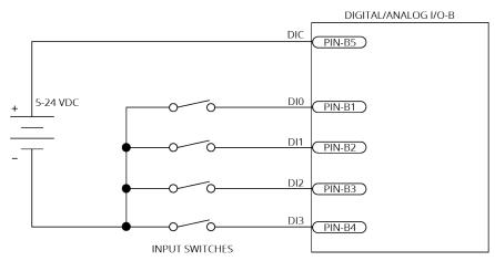
Figure 2-19: Digital Inputs Connected to Current Sinking Devices
