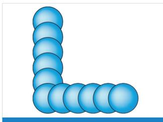
Figure 2. Laser spot placement with PSO. Notice the even overlap, even when changing direction, when Aerotech's PSO is applied. This results in consistent energy delivery and better part quality.
