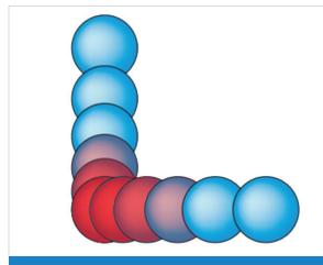
Figure 1. Laser spot placement without PSO. Notice the uneven overlap evident when changing direction which causes inconsistent energy delivery to the workpiece resulting in poor part quality.
