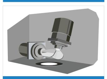
Figure 4. Aerotech's AGV Galvo Scanner where heat-dissipating electronics are removed from the scanner allowing for better thermal stability and higher-precision motion.
