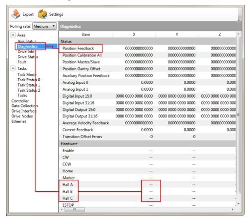
Figure 2-5: Encoder and Hall Signal Diagnostics
