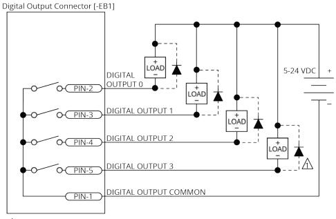
$\bigwedge$  DIODE REQUIRED ON EACH OUTPUT THAT DRIVES AN INDUCTIVE DEVICE (COIL), SUCH AS A RELAY.
