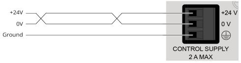
Figure 2-1: Control Supply Connections
