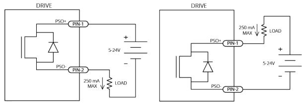
Figure 3-2: PSO Output Sources Current
