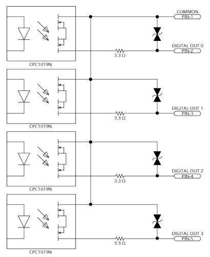
Figure 3-11: Digital Outputs Schematic [-EB1]
