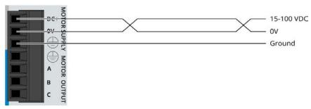
Figure 2-2: Motor Supply Connections
