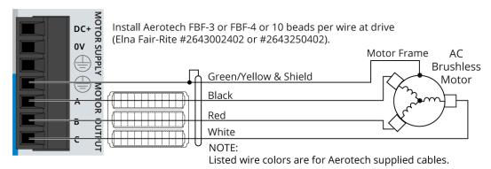
Figure 2-3: Brushless Motor Configuration
