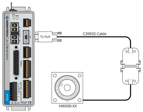
Figure 4-3: Handwheel Interconnection to the Aux Connector
