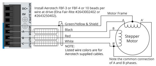
Figure 2-10: Stepper Motor Configuration
