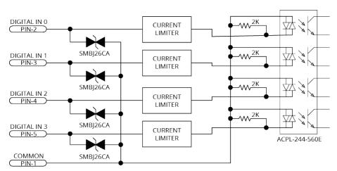
Figure 3-8: Digital Inputs Schematic [-EB1]
