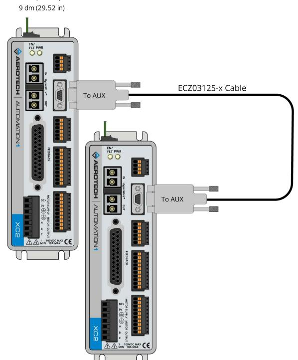
Figure 4-4: Dual-Axis PSO Cable Connection
