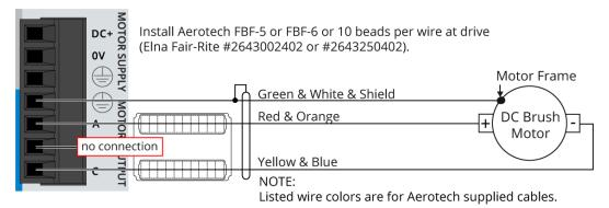
Figure 2-8: DC Brush Motor Configuration
