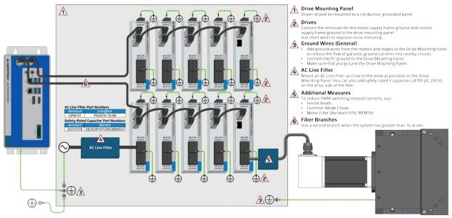
Figure 2-27: System Wiring Drawing (Best Practice)
