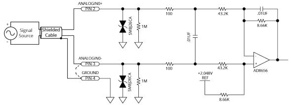
Figure 3-6: Analog Input Schematic [-EB1]
