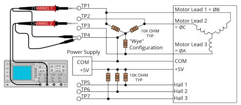
Figure 2-6: Brushless Motor Phasing Oscilloscope Example
