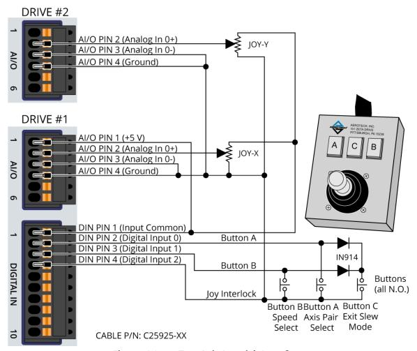
Figure 4-2: Two Axis Joystick Interface
