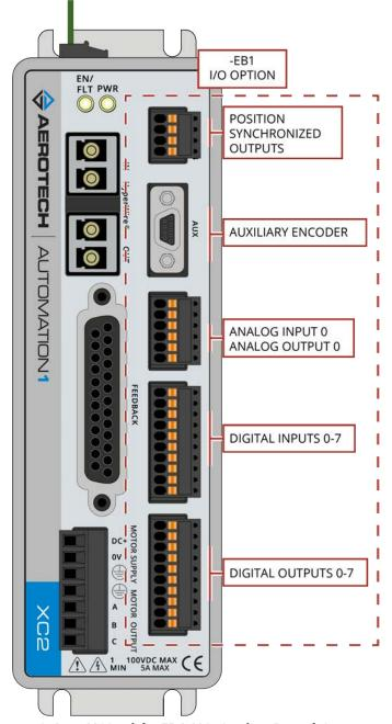
Figure 3-1: XC2 with -EB1 I/O Option Board Connectors
