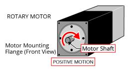
Figure 2-9: Positive Motor Direction
