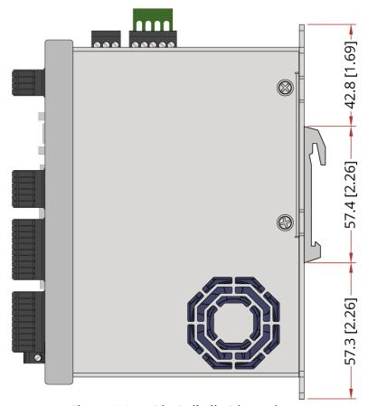
Figure 4-1: Din Rail Clip Dimensions
