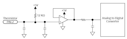
Figure 2-19: Thermistor Input Schematic (Feedback Connector)
