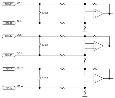
Figure 2-15: Sine Wave Encoder Schematic (Feedback Connector)
