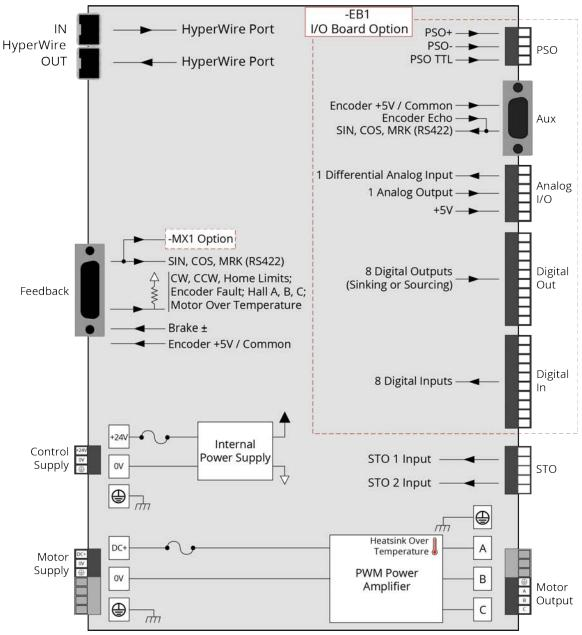
Figure 1-2: Functional Diagram
