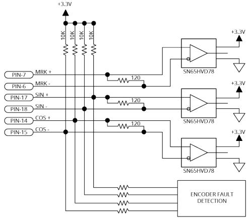
Figure 2-12: Square Wave Encoder Schematic (Feedback Connector)
