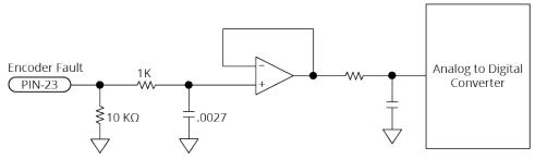
Figure 2-20: Encoder Fault Input Schematic (Feedback Connector)
