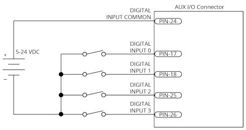
Figure 2-43: Digital Inputs Connected to Current Sinking Devices
