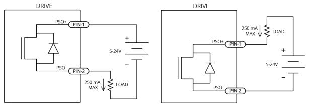
Figure 3-10: PSO Output Sources Current
