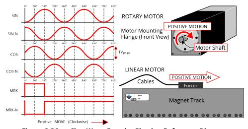
Figure 2-36: Sine Wave Encoder Phasing Reference Diagram
