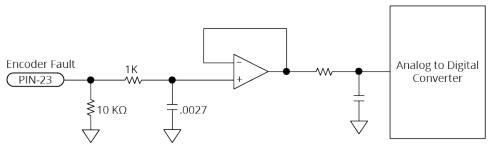
Figure 2-27: Encoder Fault Input Schematic (Feedback Connector)
