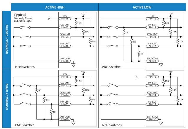
Figure 2-28: End of Travel and Home Limit Input Connections
