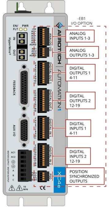
Figure 3-1: XC4e with -EB1 I/O Option Board Connectors
