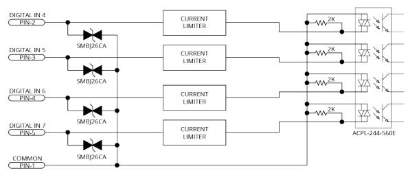
Figure 3-5: Digital Inputs Schematic [-EB1]
