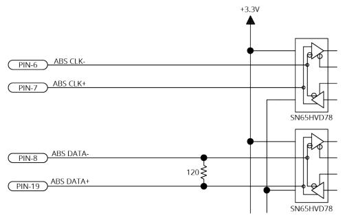
Figure 2-20: Absolute Encoder Schematic (Feedback Connector)
