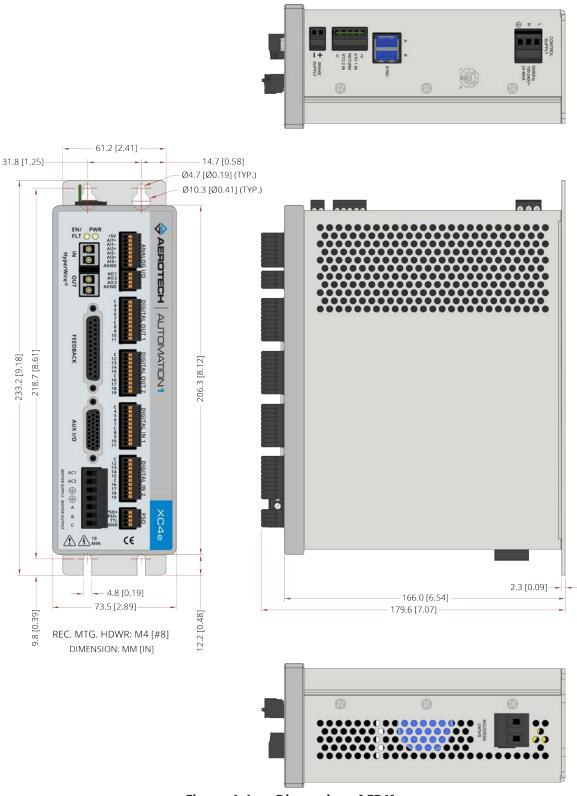
Figure 1-4: Dimensions [-EB1]
