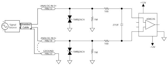
Figure 2-47: Analog Input 0 Schematic
