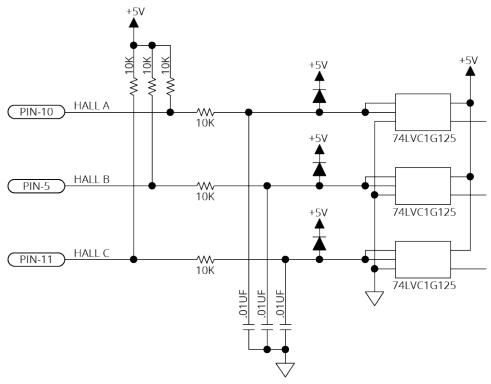
Figure 2-25: Hall-Effect Inputs Schematic (Feedback Connector)
