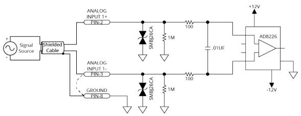
Figure 3-9: Analog Input Typical Connection [-EB1]
