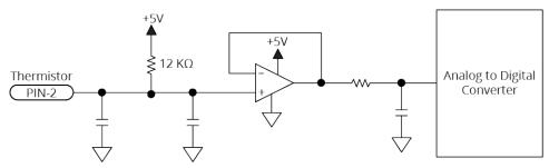
Figure 2-26: Thermistor Input Schematic (Feedback Connector)
