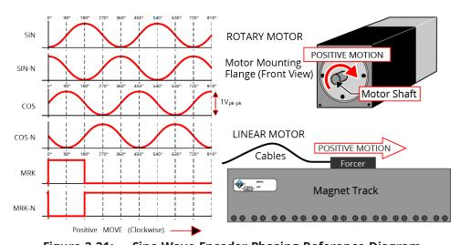
Figure 2-21: Sine Wave Encoder Phasing Reference Diagram
