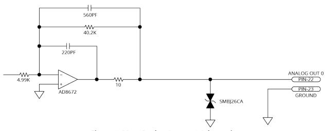
Figure 2-46: Analog Output 0 Schematic
