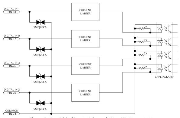
Figure 2-42: Digital Inputs Schematic (Aux I/O Connector)
