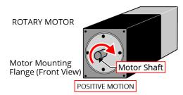
Figure 2-16: Positive Motor Direction
