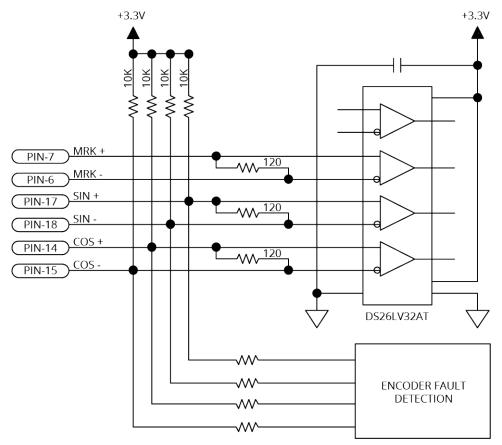
Figure 2-19: Square Wave Encoder Schematic (Feedback Connector)
