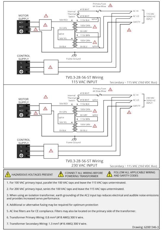
Figure 2-6: TV0.3-28-56-ST Transformer Control and Motor Power Wiring (160 VDC Bus)
