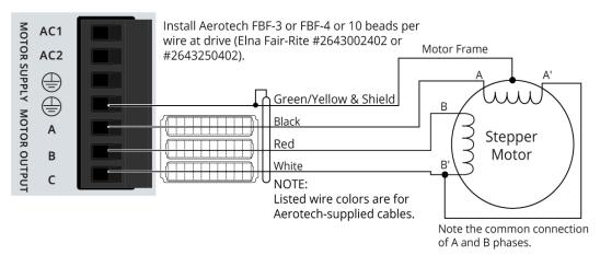
Figure 2-17: Stepper Motor Configuration
