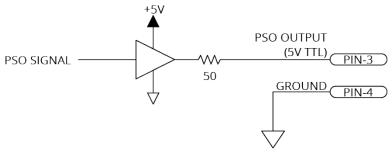
Figure 3-12: PSO TTL Outputs Schematic
