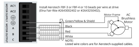
Figure 2-10: Brushless Motor Configuration
