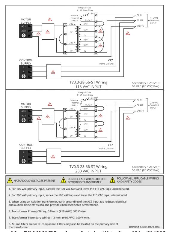
Figure 2-5: TV0.3-28-56-ST Transformer Control and Motor Power Wiring (80 VDC Bus)
