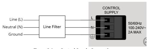
Figure 2-1: Control Supply Connections
