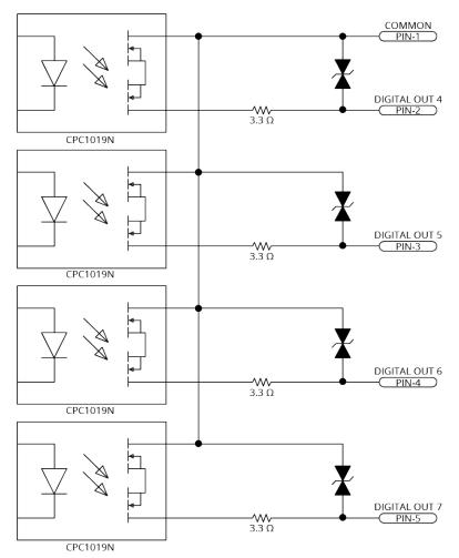
Figure 3-2: Digital Outputs Schematic [-EB1]
