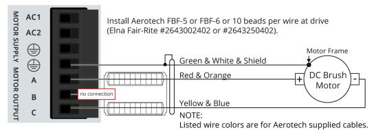
Figure 2-15: DC Brush Motor Configuration
