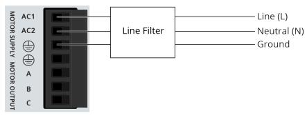
Figure 2-2: Motor Supply Connections
