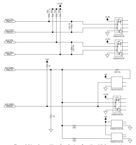
Figure 2-34: Square Wave Encoder Interface (Aux I/O Connector)
