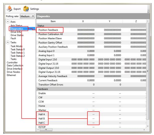
Figure 2-12: Encoder and Hall Signal Diagnostics
