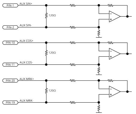
Figure 2-37: Sine Wave Encoder Schematic (Auxiliary I/O Connector)
