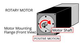
Figure 2-18: Positive Motor Direction
