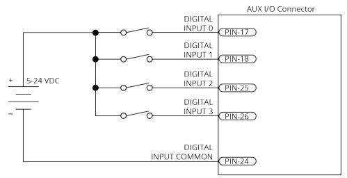
Figure 2-44: Digital Inputs Connected to Current Sourcing Devices
