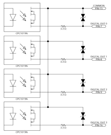
Figure 2-39: Digital Output Schematic (Aux I/O Connector)
