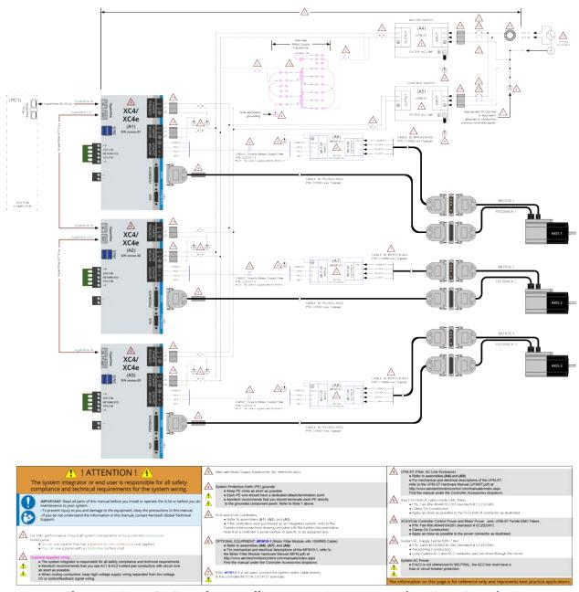
Figure 2-49: PC-Based Controller System Interconnection (Best Practice)
