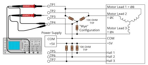
Figure 2-13: Brushless Motor Phasing Oscilloscope Example
