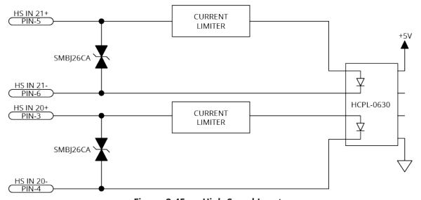
Figure 2-45: High-Speed Inputs
