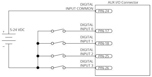
Figure 2-31: Digital Inputs Connected to Current Sinking Devices
