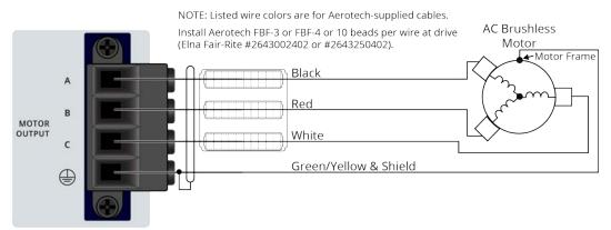
Figure 2-3: Brushless Motor Configuration
