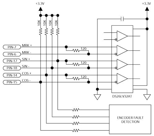
Figure 2-8: Square Wave Encoder Schematic (Feedback Connector)
