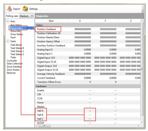
Figure 2-5: Encoder and Hall Signal Diagnostics
