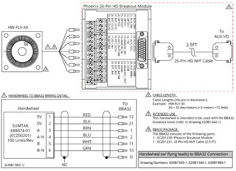
Figure 4-4: Handwheel Interconnection to the Aux I/O through a BBA32 Module
