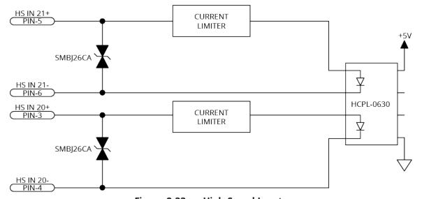
Figure 2-33: High-Speed Inputs
