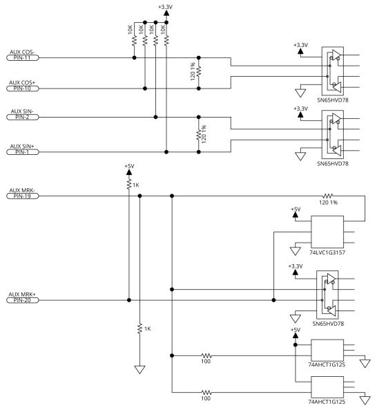
Figure 2-23: Square Wave Encoder Interface (Aux I/O Connector)
