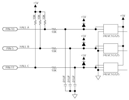
Figure 2-14: Hall-Effect Inputs Schematic (Feedback Connector)
