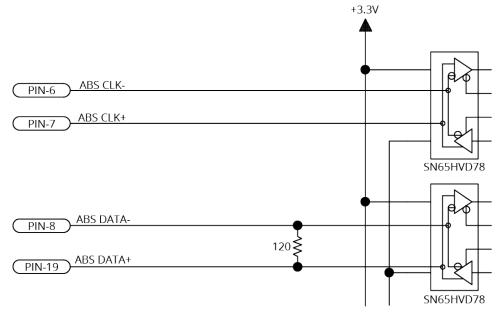
Figure 2-9: Absolute Encoder Schematic (Feedback Connector)
