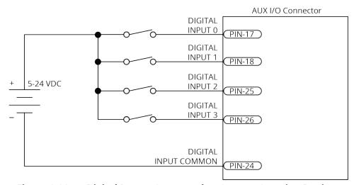
Figure 2-32: Digital Inputs Connected to Current Sourcing Devices
