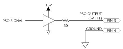
Figure 3-12: PSO TTL Outputs Schematic
