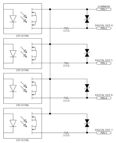
Figure 3-2: Digital Outputs Schematic [-EB1]
