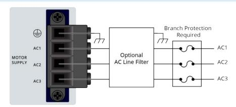
Figure 2-2: Motor Supply Connections
