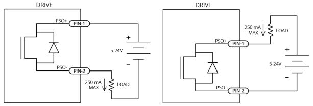
Figure 3-10: PSO Output Sources Current
