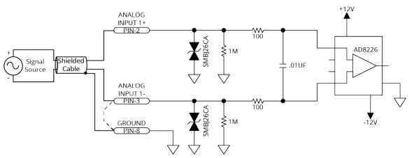
Figure 3-9: Analog Input Typical Connection [-EB1]
