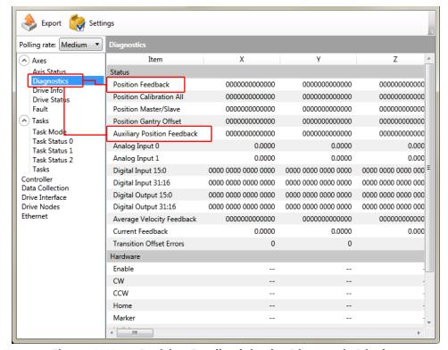
Figure 2-13: Position Feedback in the Diagnostic Display
