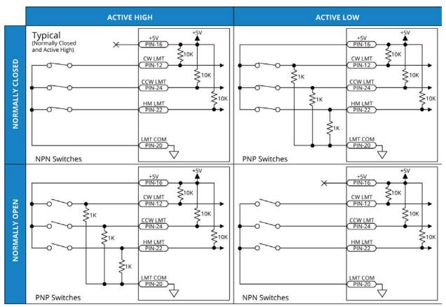
Figure 2-17: End of Travel and Home Limit Input Connections
