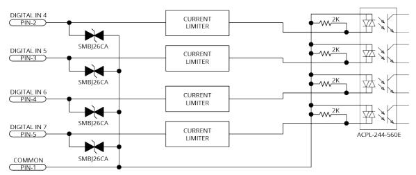
Figure 3-5: Digital Inputs Schematic [-EB1]
