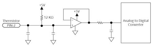
Figure 2-15: Thermistor Input Schematic (Feedback Connector)
