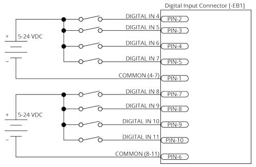
Figure 3-6: Digital Inputs Connected to Current Sourcing (PNP) Devices [-EB1]
