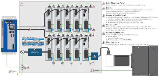
Figure 2-36: System Wiring Drawing (Best Practice)
