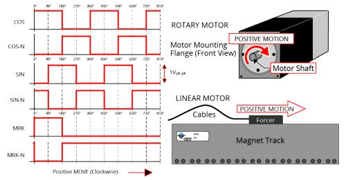
Figure 2-12: Encoder Phasing Reference Diagram (Standard)
