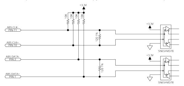
Figure 2-24: Absolute Encoder Schematic (Auxiliary I/O Connector)
