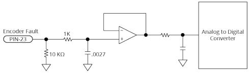
Figure 2-16: Encoder Fault Input Schematic (Feedback Connector)
