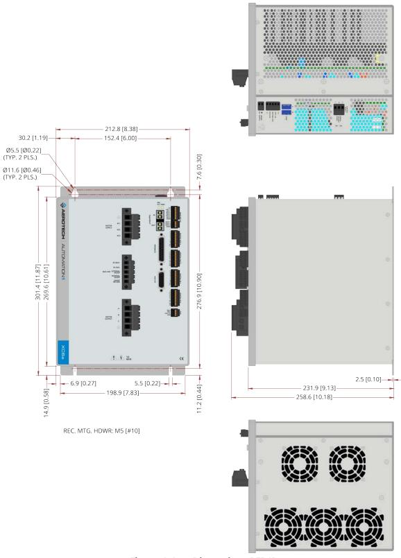
Figure 1-4: Dimensions [-EB1]
