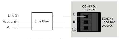
Figure 2-1: Control Supply Connections
