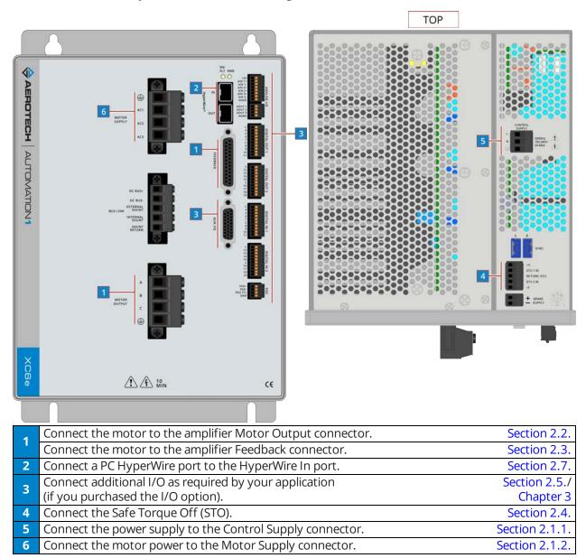
Figure 1: Installation Connection Overview
