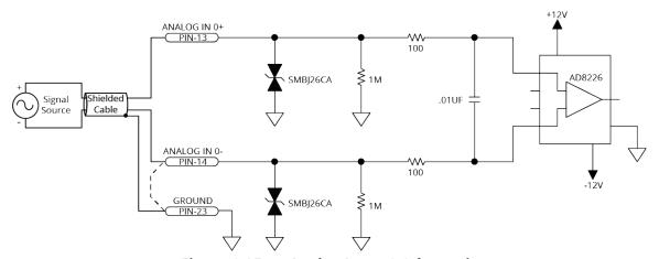
Figure 2-35: Analog Input 0 Schematic
