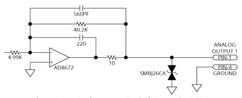
Figure 3-8: Analog Output Typical Connection [-EB1]
