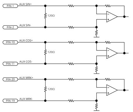
Figure 2-26: Sine Wave Encoder Schematic (Auxiliary I/O Connector)
