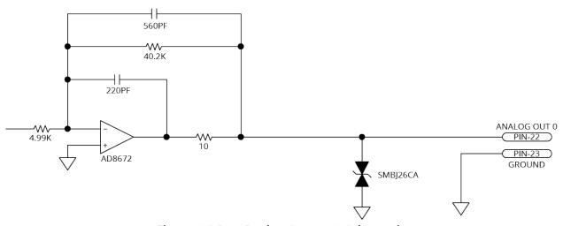
Figure 2-34: Analog Output 0 Schematic
