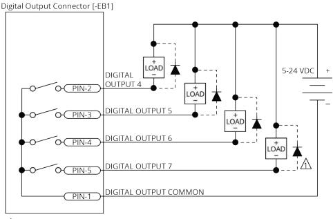
DIODE REQUIRED ON EACH OUTPUT THAT DRIVES AN INDUCTIVE DEVICE (COIL), SUCH AS A RELAY.
