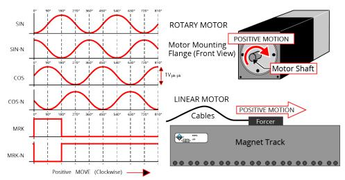
Figure 2-10: Sine Wave Encoder Phasing Reference Diagram
