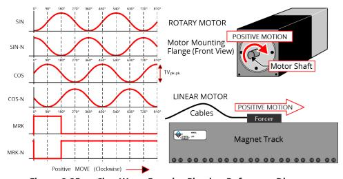
Figure 2-25: Sine Wave Encoder Phasing Reference Diagram
