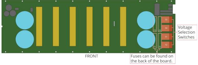
Figure 3-1: Drive Interface Board
