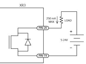
Figure 2-25: PSO Output Sinks Current
