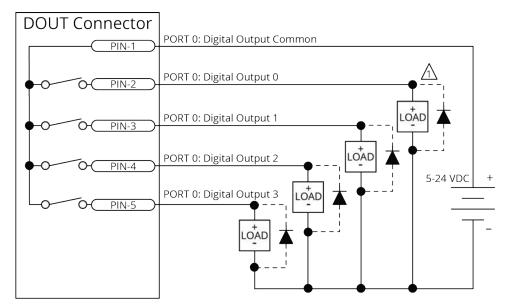
$\Lambda$  Diode required on each output that drives an inductive device (coil), such as a relay.
