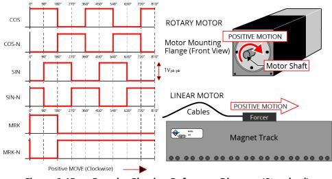
Figure 2-15: Encoder Phasing Reference Diagram (Standard)
