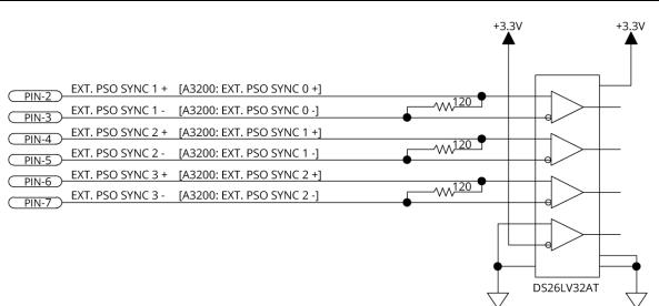
**Figure 2-27: PSO Clock Inputs Schematic**
