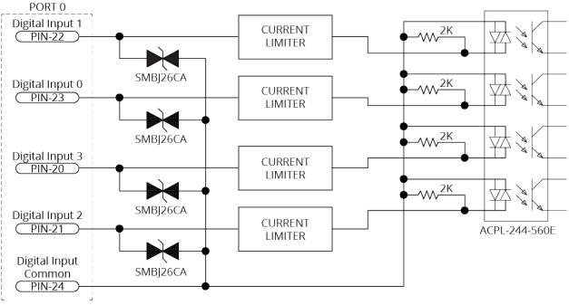
Figure 2-33: Digital Input Schematic
