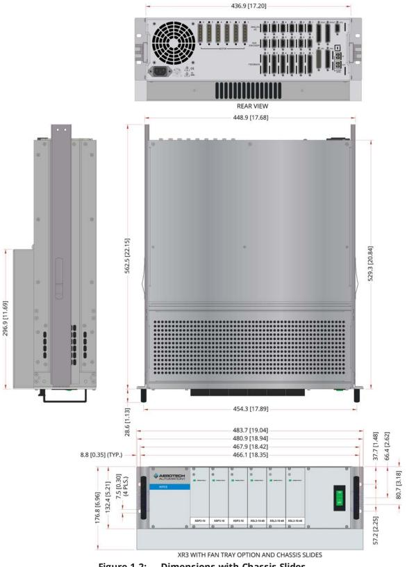
Figure 1-2: **Dimensions with Chassis Slides**
