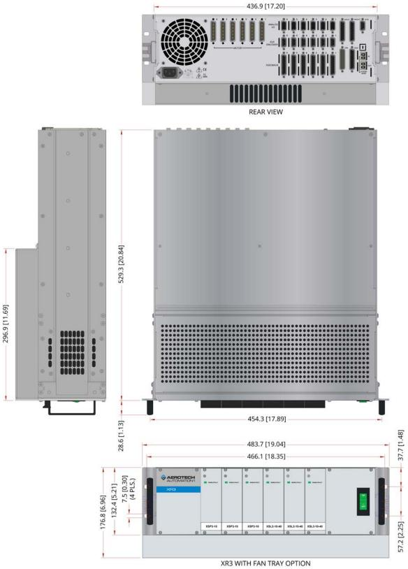
Figure 1-3: Dimensions without Chassis Slides
