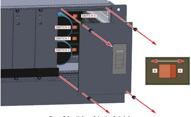
Figure B-1: Voltage Selection Switch Access
