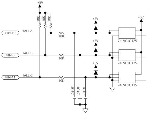
**Figure 2-17:** Hall-Effect Inputs Schematic (Feedback Connector)
