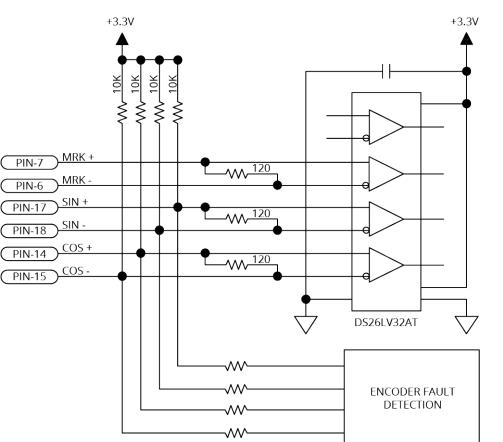
Figure 2-11: Square Wave Encoder Schematic (Feedback Connector)
