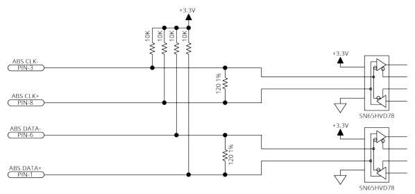
Figure 2-37: Absolute Encoder Schematic (Aux Encoder Connector)
