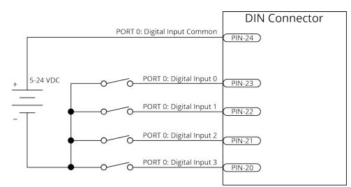
Figure 2-34: Digital Inputs Connected to Current Sinking (NPN) Devices
