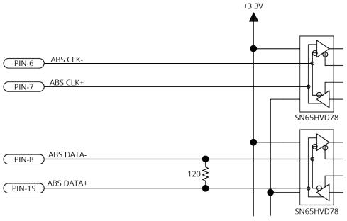
Figure 2-12: Absolute Encoder Schematic (Feedback Connector)
