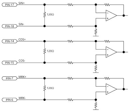
Figure 2-14: Sine Wave Encoder Schematic (Feedback Connector)
