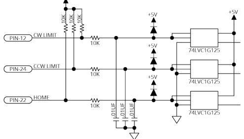
Figure 2-21: End of Travel and Home Limit Input Schematic (Feedback Connector)
