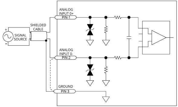
Figure 2-41: Analog Inputs Schematic
