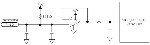
Figure 2-18: Thermistor Input Schematic (Feedback Connector)
