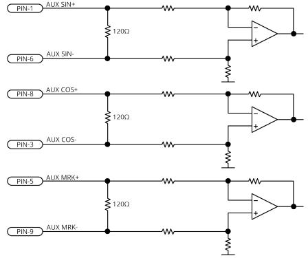
Figure 2-39: Sine Wave Encoder Schematic (Aux Encoder Connector)
