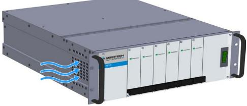
Figure 2-47: -C0 Fan Location and Direction of Air Flow
