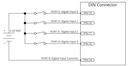
Figure 2-35: Digital Inputs Connected to Current Sourcing (PNP) Devices
