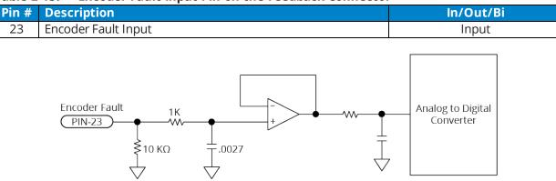
Figure 2-19: Encoder Fault Input Schematic (Feedback Connector)
