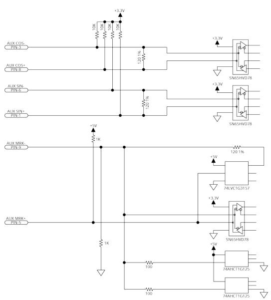
Figure 2-36: Square Wave Encoder Interface (Aux Encoder Connector)
