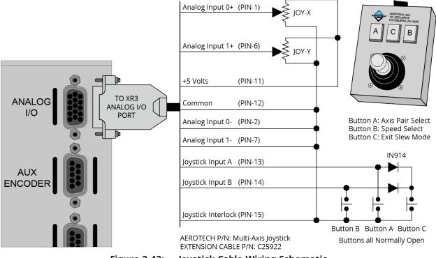
Figure 2-43: Joystick Cable Wiring Schematic
