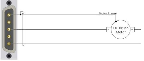
Figure 2-7: DC Brush Motor Configuration
