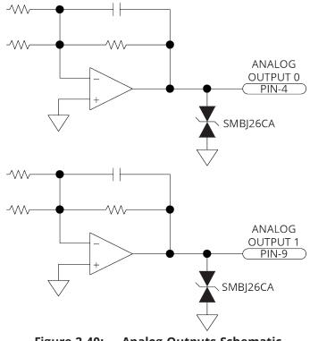
Figure 2-40: Analog Outputs Schematic
