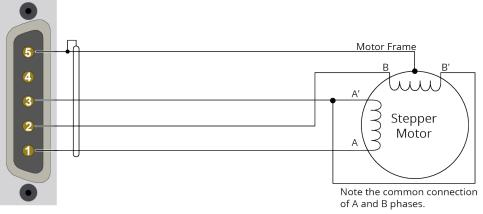
Figure 2-9: Stepper Motor Configuration
