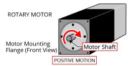
Figure 2-8: Positive Motor Direction
