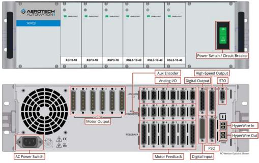
Figure 2-1: Power and Control Connections
