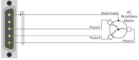
Figure 2-2: Brushless Motor Configuration
