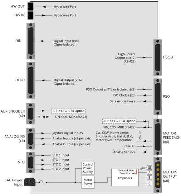
Figure 1-1: Functional Diagram
