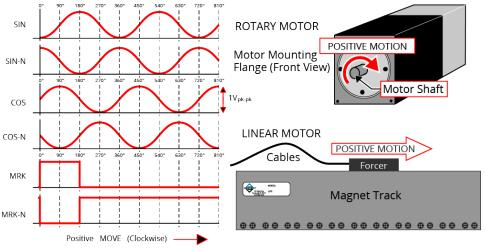
Figure 2-13: Sine Wave Encoder Phasing Reference Diagram
