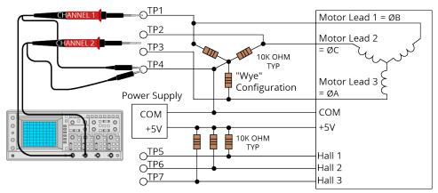
Figure 2-5: Brushless Motor Phasing Oscilloscope Example
