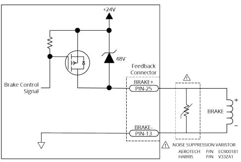
Figure 2-23: Brake Output Connections (Feedback Connector)
