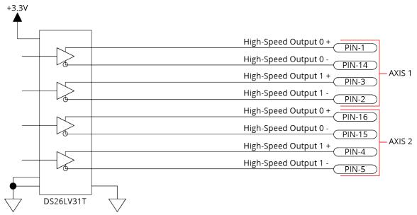
Figure 2-29: Diagram Showing Axis 1 and Axis 2 High-Speed Outputs
