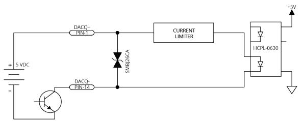
Figure 2-28: Data Acquisition Input Schematic
