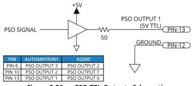
Figure 2-26: PSO TTL Outputs Schematic
