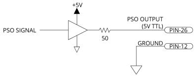
Figure 2-21: PSO TTL Outputs Schematic
