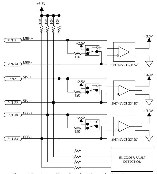
Figure 2-9: Square Wave Encoder Schematic (Axis Connector)
