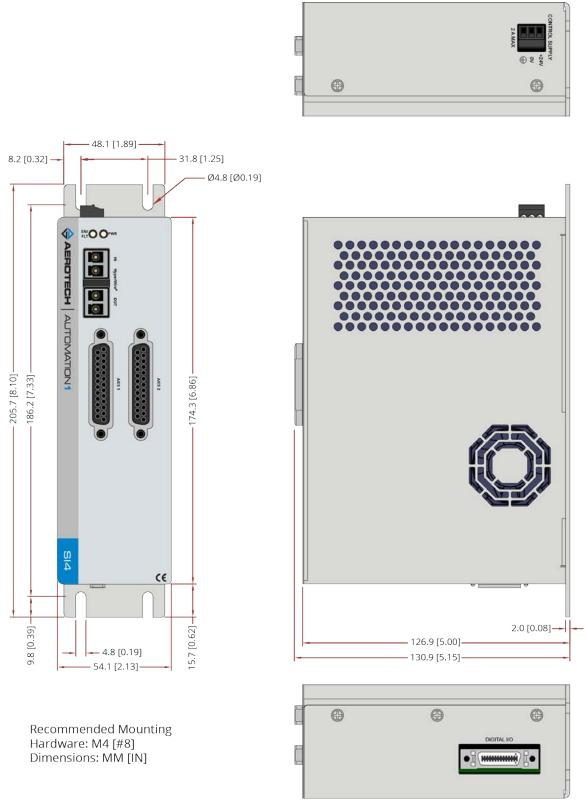
Figure 1-4: Dimensions [-2P1 (Standard 2-Axis)]
