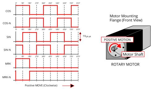
Figure 2-11: Encoder Phasing Reference Diagram (Standard)
