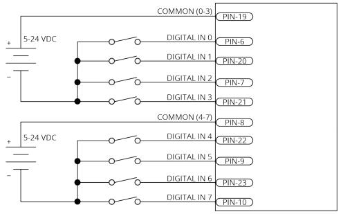
Figure 2-16: Digital Inputs Connected to Current Sinking (NPN) Devices
