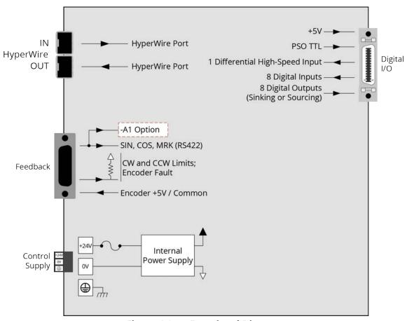
Figure 1-3: Functional Diagram
