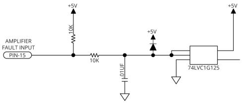
Figure 2-7: Fault Input Schematic
