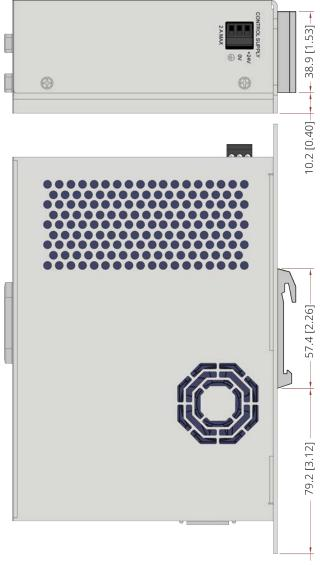
Figure 1-8: Din Rail Clip Dimensions
