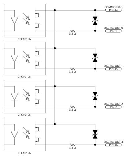
Figure 2-17: Digital Outputs Schematic
