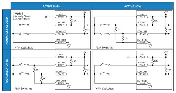
Figure 2-4: End of Travel Limit Input Connections
