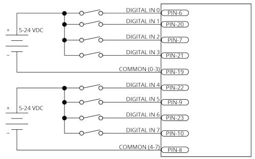
Figure 2-15: Digital Inputs Connected to Current Sourcing (PNP) Devices
