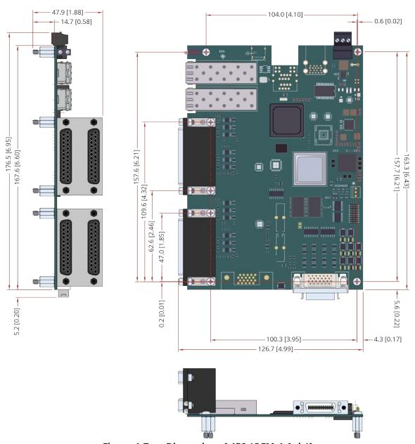
Figure 1-7: Dimensions [-4P2 (OEM 4-Axis)]
