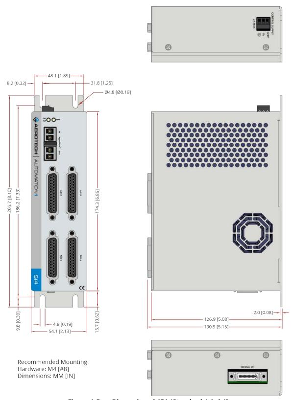
Figure 1-5: Dimensions [-4P1 (Standard 4-Axis)]
