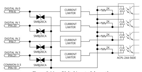
Figure 2-14: Digital Inputs Schematic
