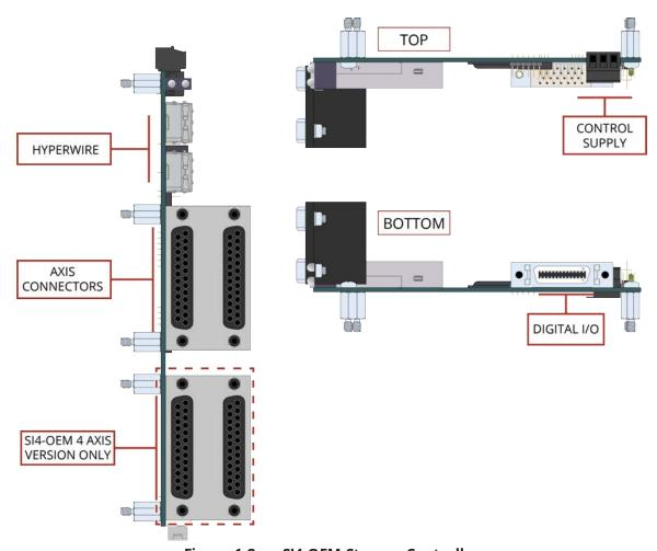
Figure 1-2: SI4-OEM Stepper Controller
