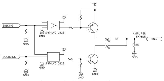
Figure 2-8: Amplifier Enable Output Schematic
