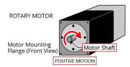
Figure 2-13: Positive Motor Direction
