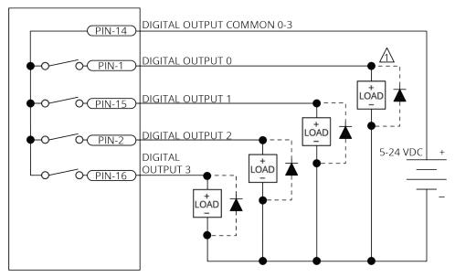
$\bigwedge$  DIODE REQUIRED ON EACH OUTPUT THAT DRIVES AN INDUCTIVE DEVICE (COIL), SUCH AS A RELAY.
