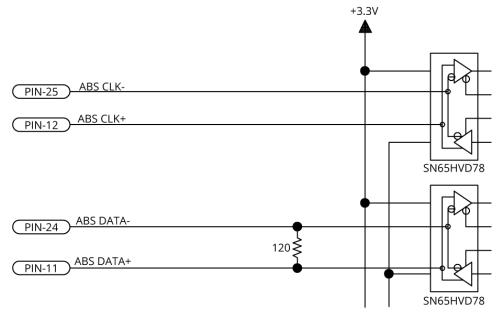
Figure 2-10: Absolute Encoder Schematic (Axis Connector)
