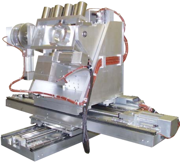
Optics Polishing System. Custom, multi-axis, high-vacuum system using a variety of staging technologies.
