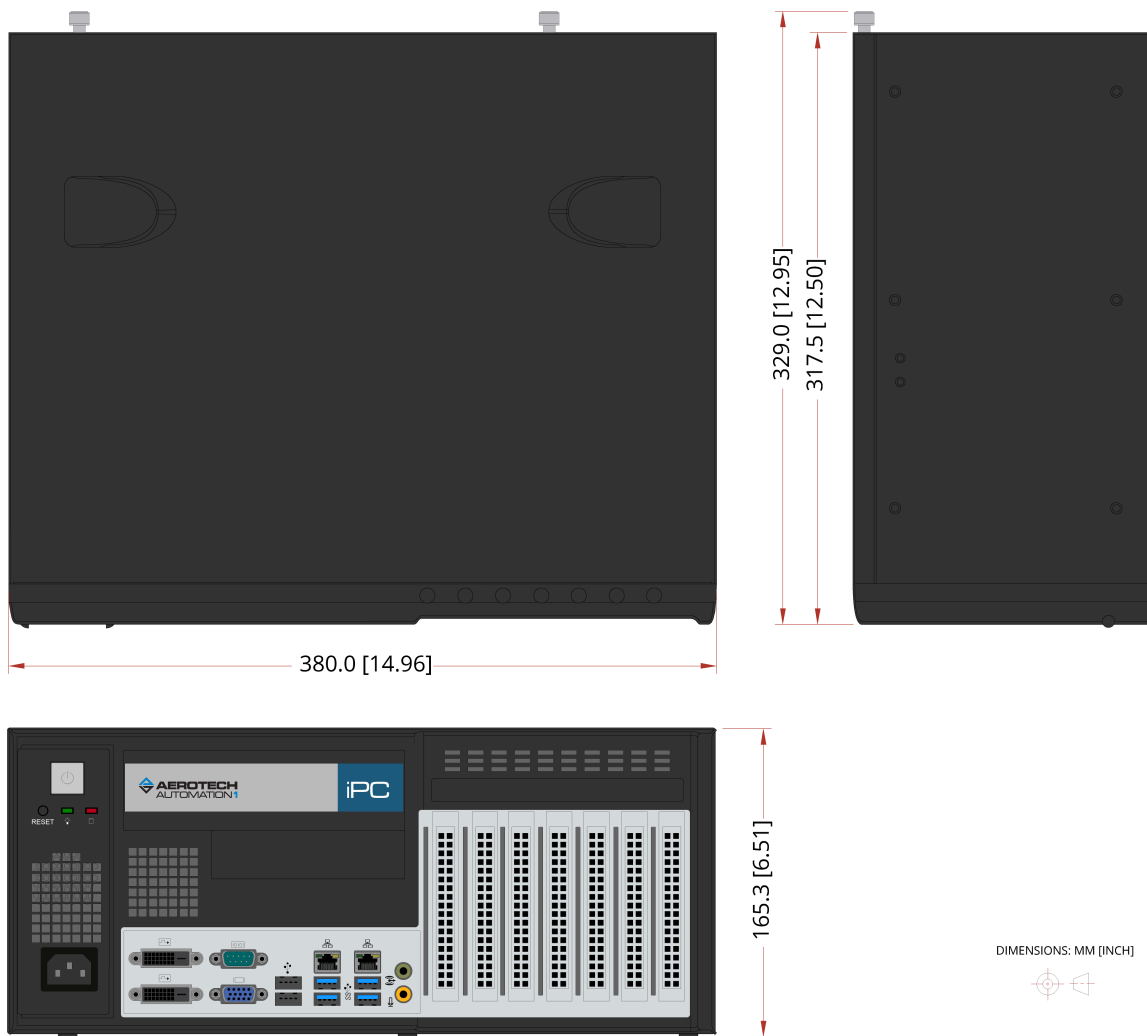
Figure 1-5: Desktop Computer Dimensions (-DT01)
